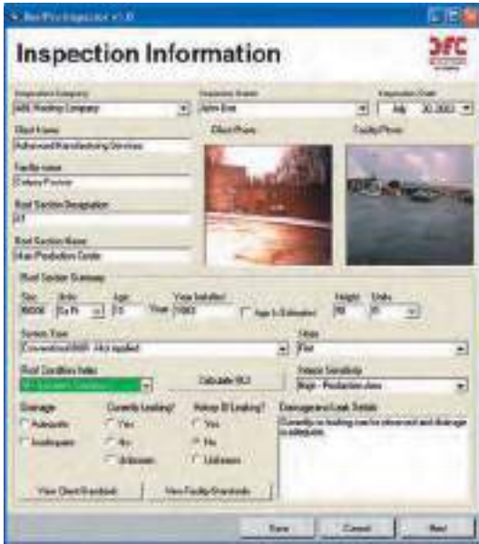
Roof inspectors can enter data while on the roof using tablet computers. Digital cameras allow inspectors to easily and quickly take photographs of problems areas. These photographs, as well as information stored on the tablet PC, can then be downloaded directly into a database when the inspectors return to their offices, eliminating several steps in the collection process.
